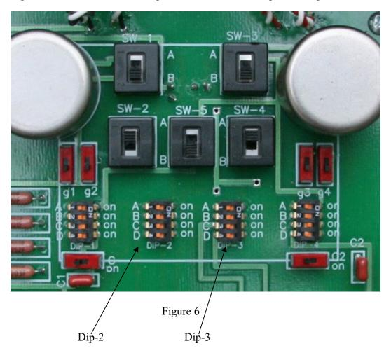
Switches SW1, SW3, and SW-5 should all be switched to the forward position. Switches SW2 and SW4 should be switched toward the rear as shown in figure 6. Dip –2 and Dip-3 are used to set the cartridge loading according to the following table:
