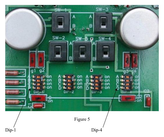
Switches SW1, SW2, SW3, SW4 and SW-5 should all be switched to the rear. Dip –1 and Dip-4 are used to set the cartridge loading according to the following table:
