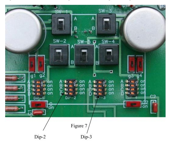
Switches SW1, SW2,SW3, SW4 and SW-5 should all be switched to the forward position as shown in figure 7.
